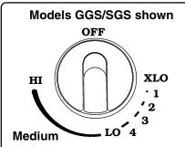
All the controls have an infinite number of heat settings, with no fixed positions between HI, LO or XLO. The word (Medium) and number designations are for reference only and are guides to the flame settings referenced in the following chart.
